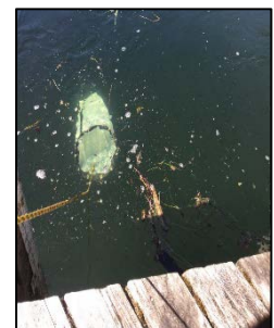
Figure 33. Plankton tow net used to sample for Dreissenid veligers (larvae).
